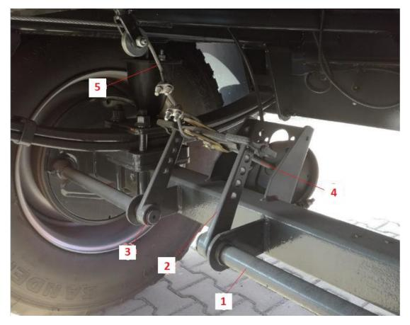
Fig. 20. Brake system components: 1– shoe spreader shaft, 2 – spreader shaft lever (arm), 3 – arm adjustment "comb" on the spreader shaft, 4 - tie (push) rod connecting the piston rod of the pneumatic actuator with the spreader shaft arm, 5 – parking brake line.
